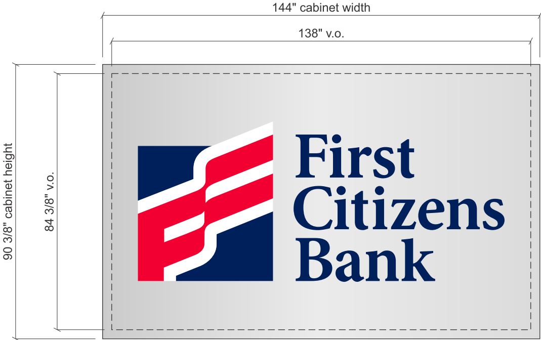
1 Pylon Sign Face Replacements - Front View Scale: 3/8" = 1'-0"
